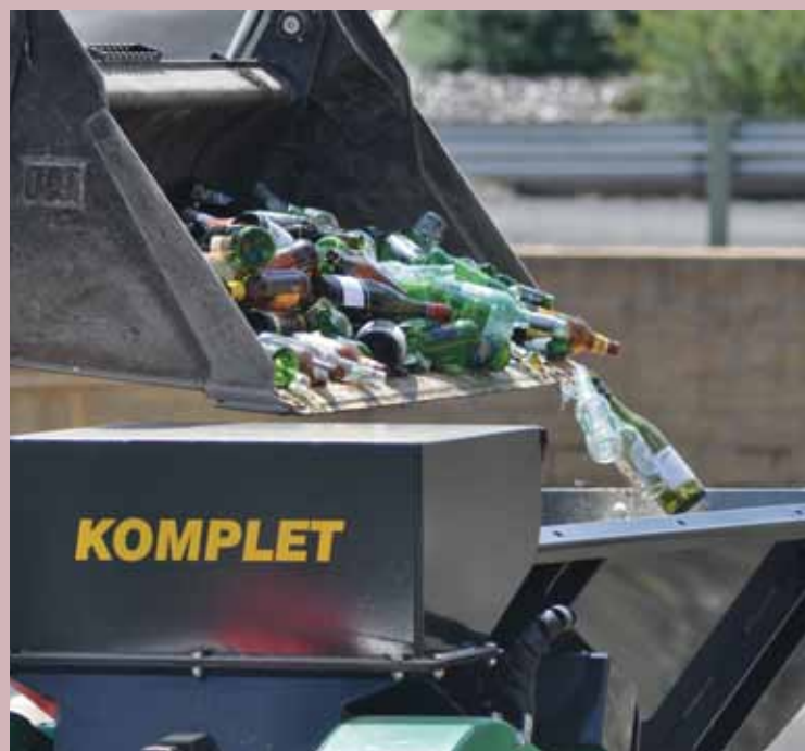
Glass being tipped into the crusher, output from the glass crusher
